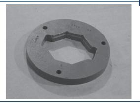
Select the corresponding Thrust Plate for the size fitting you are installing. Assuring that the recess is facing outward toward the operator, slide the Thrust Plate over the Pull Rod until it reaches the **25ROSTPA**. Align the holes in the Thrust Plate with the dowel pins on the **25ROSTPA** and slide the Thrust Plate over the pins. Tighten the wing nut to lock in place.
