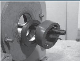
Install the **001-0067** into the Master IX Adapter opening and secure with Adapter Straps (**25ROSTPA**) and two  $\frac{1}{2}$ " - 13 UNC Hex Bolts 15%" long.
