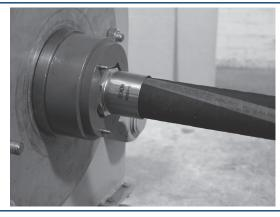
While holding the hose and ferrule firmly against the stem shoulder, engage the ram cylinder by stepping on the foot pedal (or depressing the "ON" button on the remote control.) The internal expansion operation is complete when the hose and stem assembly is pushed completely over the internal expansion plug. Releas the foot pedal or "ON" switch.
