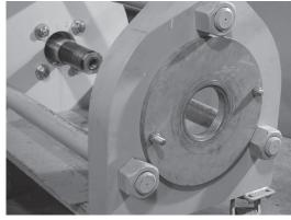
Install the Master IX Adapter (50T-0072) into the Die Bed Plate (50T001). Secure in place using two Adapter Straps (001-0072A) and  $\frac{3}{4}$ " - 10 UNC x 8" rods.
