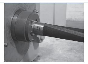
Slide the hose with the ferrule on over the shank until the ferrule contacts the shoulder of the stem. Make sure you align the ferrule with the second mark from step 8. Make sure the pocket has been maintained.
