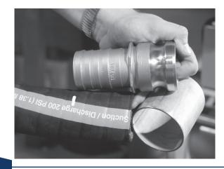
Place a mark on the outside of the ferrule that corresponds with the center of one of the turned over sections of the ferrule. This mark will act as a guide for correct engagement with the stem collar.
