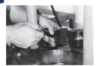
Lubricate the I.D. of both die halves with Crisco<sup>®</sup> (recommended) or high viscosity oil or heavy duty grease.
