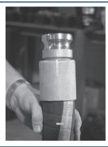
Bring the hose with the stem and ferrule through the die bed. Insert the coupling into or onto the pusher (depending upon coupling style). Make sure that there is sufficient room between the die holders and the end of the ferrule to comfortably insert the die halves into the die holders.
