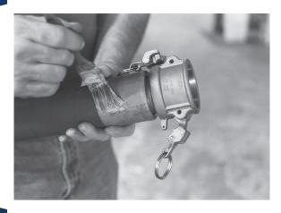
Lubricate the outside of the ferrule with Crisco<sup>®</sup> (recommended) or high viscosity oil or heavy duty grease.
