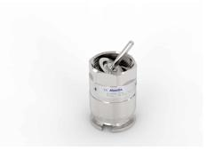
Refit the spring (pos.7), bushing (pos.5) and piston guide (pos.4).
