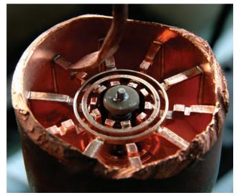
A magnetron creates high-power electromagnetic pulses, like the ones used in microwave ovens or radar systems. *Photo: Pingu Is Sumerian*
