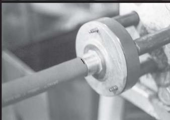
8 Holding the hose and ferrule firmly against the stem shoulder and, maintaining the proper "pocket", engage the Ram by stepping on the foot pedal. The internal expansion operation is complete when the hose and stem assembly is pushed completely over the internal expansion plug. Release the foot pedal. Visually inspect the coupling.
