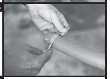
Make sure the hose end is cut square. Measure and mark the hose in accordance with the provided Insertion Dimension chart (*see page 5*). This will ensure that the proper rubber displacement "pocket" is maintained when proceeding to Step 7.
