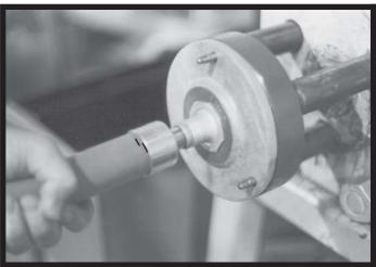
Ensuring that the end of the ferrule is aligned with the mark from Step 6, slide the hose with ferrule over the shank until the ferrule contacts the shoulder of the stem. Check to see if the proper pocket is maintained.
